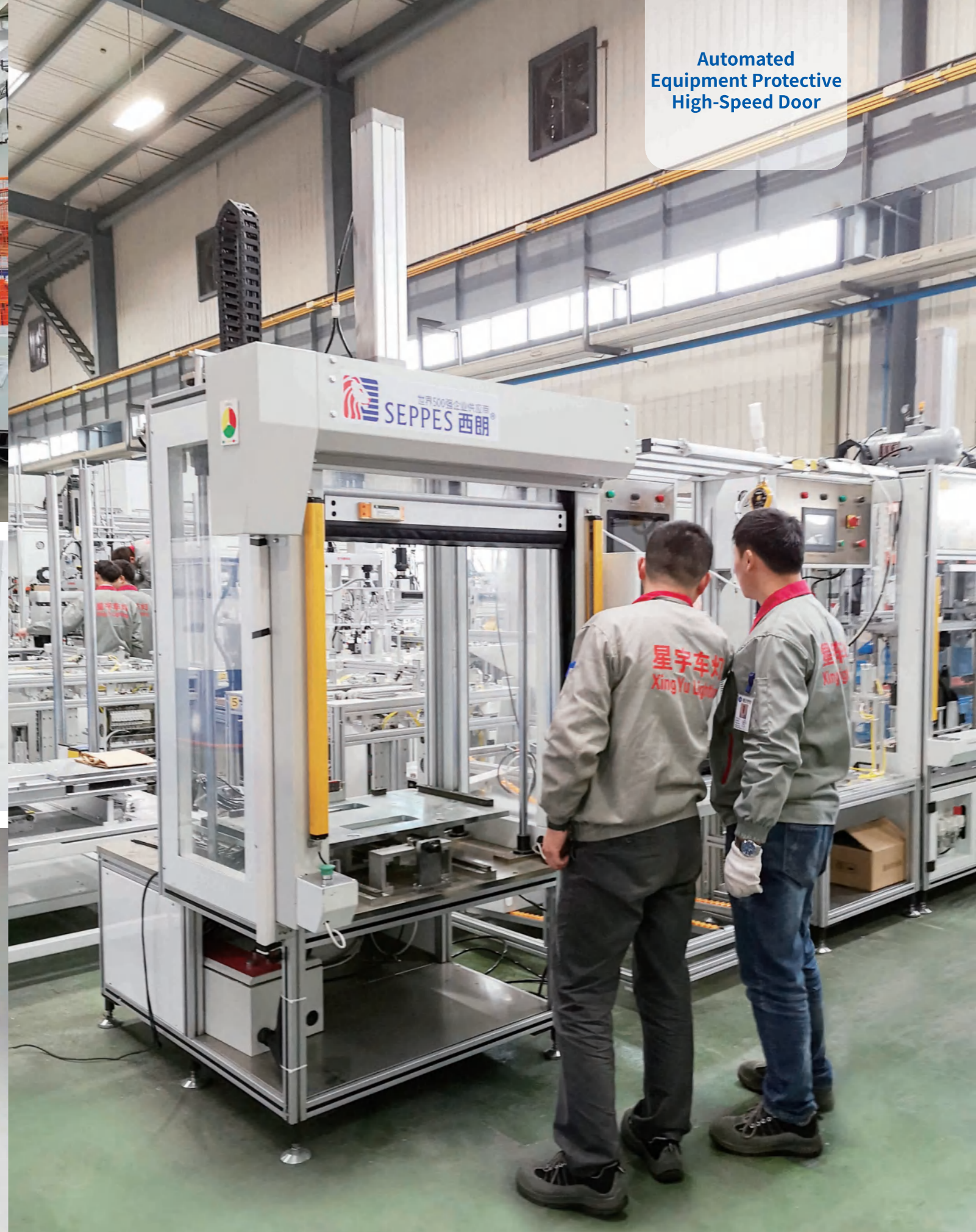
Automated Equipment Protective High-Speed Door (Xingyu Automotive Lighting)
