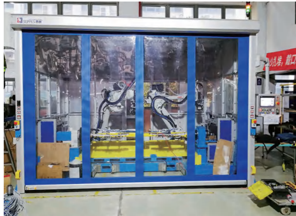
Robot Workshop Protective Door (Panoramic Window)
